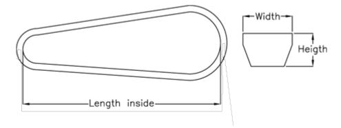
$\begin{array}{ll} \text{Datum Llength} = 735 \\ \text{Height} &= 10 \\ \text{Length inside} &= 695 \\ \text{Width} &= 17 \end{array}$
